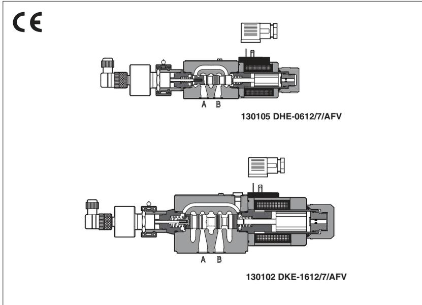
Directional safety valves specifically designed for applications in vertical presses and torque bar press brakes, are provided with ON-OFF inductive position switch FV (double contacts NC/NO) indicating the position of the valve's spool
