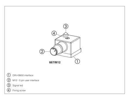
Electric connectors with standard DIN 43650 solenoid interface and M12, 5 pin interface to the user side.
