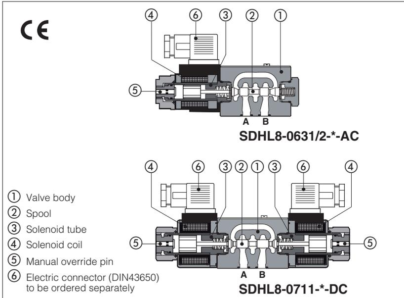
Spool type, two or three position direct operated solenoid valves size 06 **in low leakage and compact execution** with reduced solenoids dimensions, ideal for hydraulic systems assisted by accumulators.
