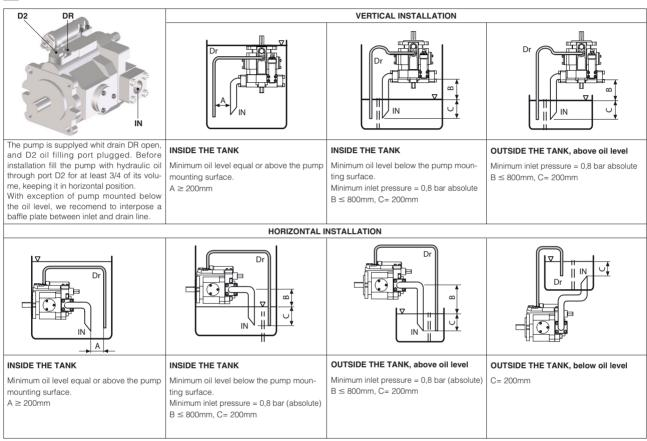
IN: inlet line - DR: drain line - A: minimum distance between inlet and drain line - B+C: permissible suction height - C: inlet line immersion depth
