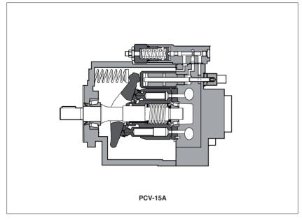
PVC are variable displacement axial piston pumps for medium pressure operation, low noise level, suitable for open circuit systems.
