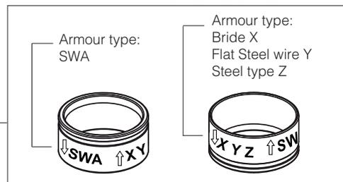
**Note:** the arrow corresponding to the correct armour type (SWA or X, Y, Z) must be oriented towards the ex-proof solenoid
