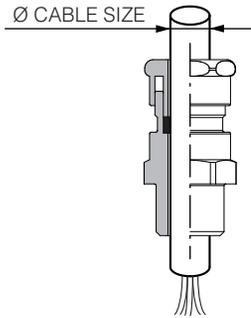
Cable glands for use with non-armoured plastic insulated cables
